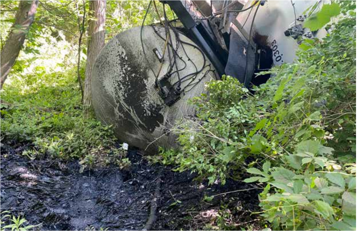
Overturned tanker spilling asphalt emulsion that would eventually reach the Ferdon Intercounty Drain.
