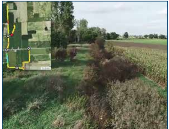
BL DENMAN Enterprises utilizes UAV overflight of drains to obtain visual inventory of vegetation conditions of county drains
