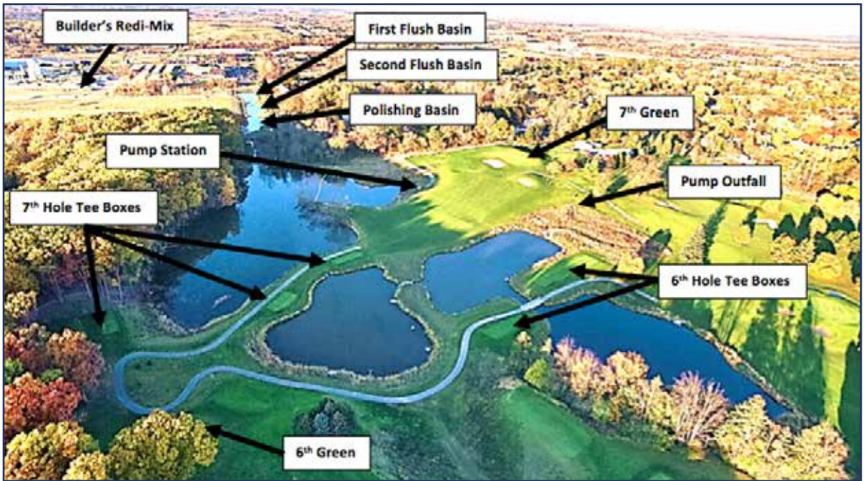
Aerial view overlooking the golf course, storm water detention storage and water quality improvement features
